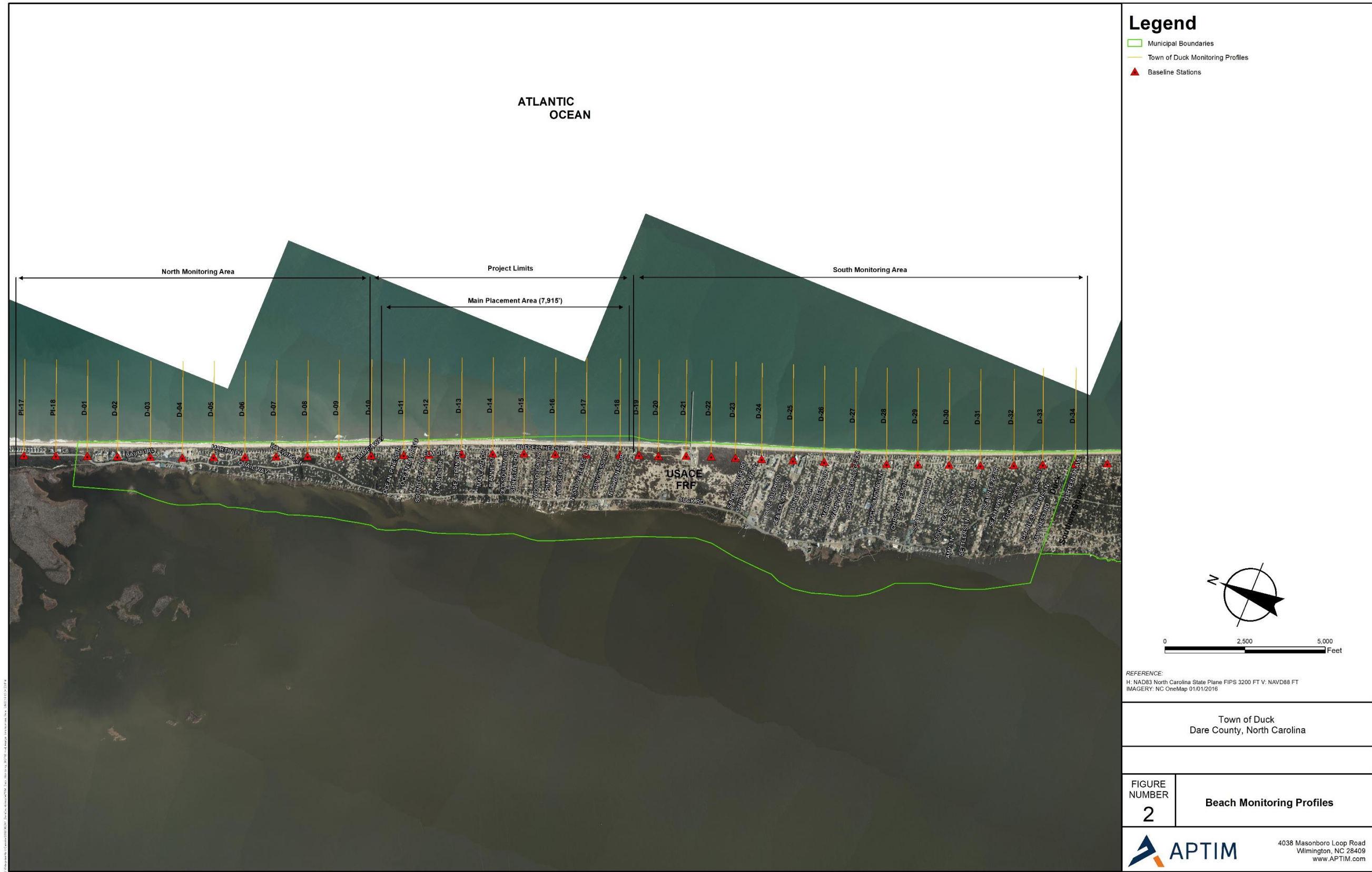
Figure 2. Detailed project area map showing the Project Area, North Monitoring Area, South Monitoring Area, and the location of the monitoring profiles.
